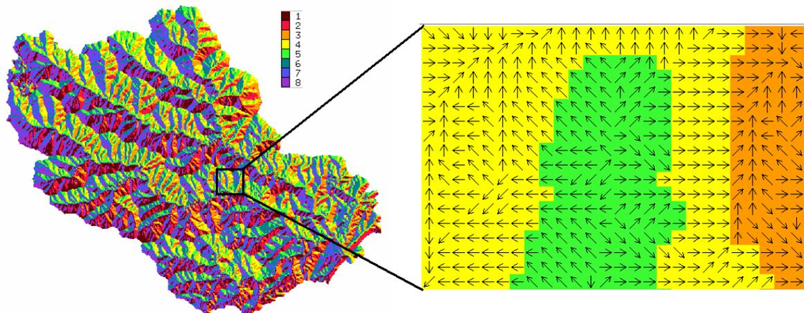
Figure 2-10 : Drainage pathways of each cell of the catchment. A given cell flows towards the neighboring cell which has the lowest elevation
