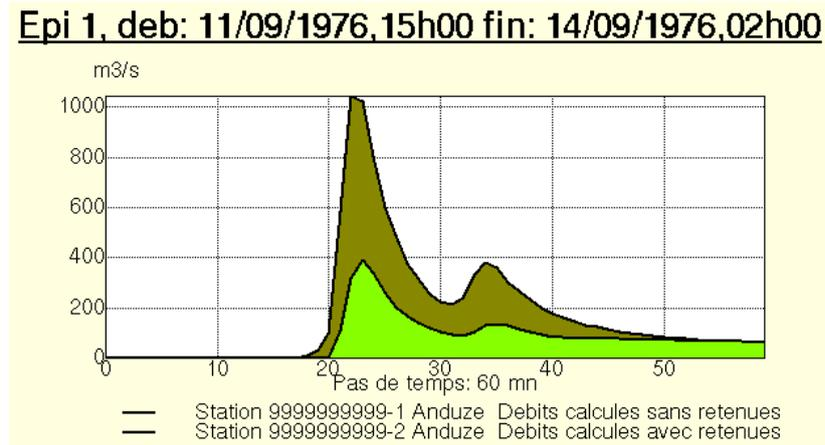
*Figure 5-7 : Discharges at Anduze with or without reservoirs.*
